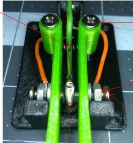
3/4 inch screw for ground. Attach the green or white wire to the bottom of the screw on the under side of the base
