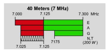
Depending on height of antenna, this band gets longer (goes further) as evening sets in. NVIS (near vertical incident skywave) as the antenna gets lower to the ground. Good for state QSO parties.
